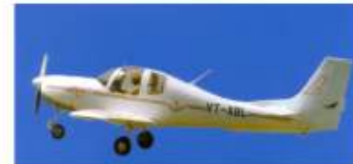
HANSA –3 (NAL's All – Composite Light Trainer Aircraft)
