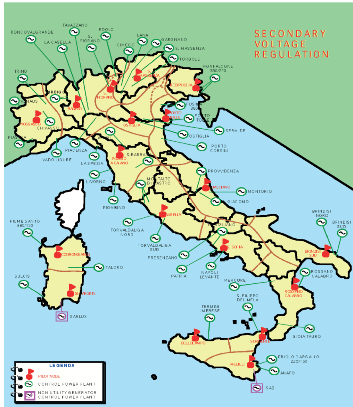
Application plan of the hierarchical Secondary Voltage Regulation in the Italian grid.
